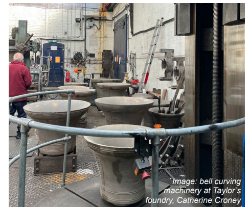
Image: bell curving machinery at Taylor's foundry, Catherine Croney
